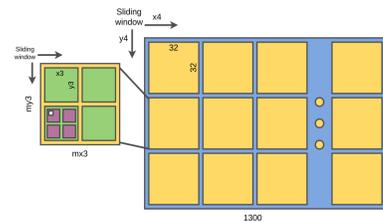
We compute a histogram of gradients within the region defined by a given kernel at a given pixel location. Points are randomly discarded at lower-gradient pixel locations if the region is dense in points. Dynamic pixel selector
